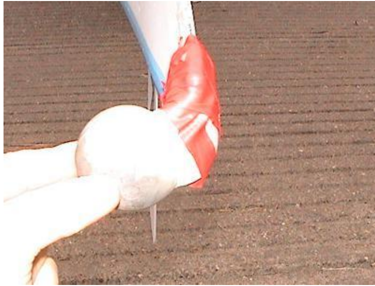
Bow Ball only taped on – Not Acceptable
