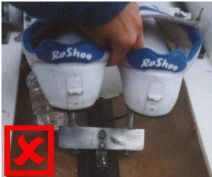
No clips for Heel Restraint – Not Acceptable
