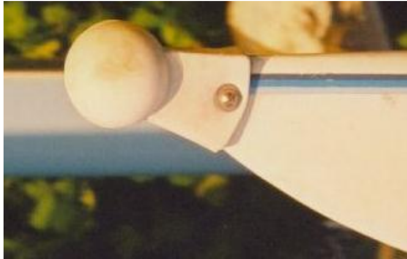
Well fitting Bow Ball – Acceptable
